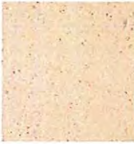
CS1 Material: Cast Stone Finish: Light Sandblast Color: to match SpecStone "Granada White" #1801
