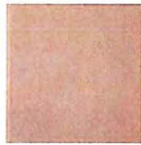
CT3 Material: Concrete Finish: Broom Color: Davis 860 "Cobblestone"
