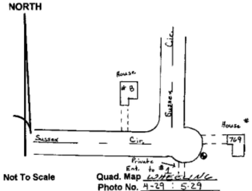
DESCRIPTION: Station is a concrete monument with a Brass Cap, located midway between Back of Curb and the Front of walk, (in Boulevard) ± 11' S/o R<sup>o</sup> Maple, ± 9' NE/o Street light.
