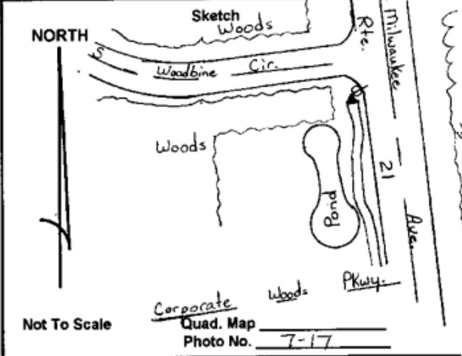
DESCRIPTION: Set a 5/8" Rebar w/ Red Cap Stamped "Ayres Assoc. G.P.S. Station" @ End of sidewalk, in center of sidewalk, Southwest Quadrant Milwaukee Av./S. Woodbine Cir.
